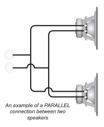
• The negative output terminal of the right channel connects to the negative input post of the first speaker **and** to the negative post of the second speaker.
